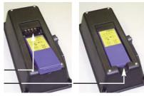
If the Hydrotector  $\mathbf{H}_{\scriptscriptstyle 2}$  cannot be turned on, check that the accumulator has been correctly installed.
