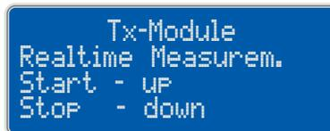
The sensors of the connected Tx-bus are polled in sequence.
