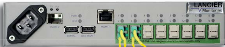
OTDR with RTU and optical switches
