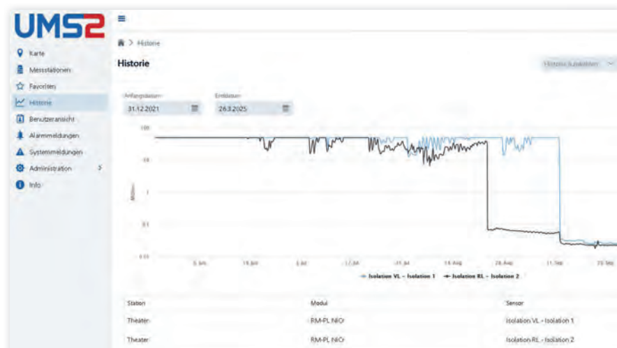
Measurement history of the insulation value of a district heating pipeline
