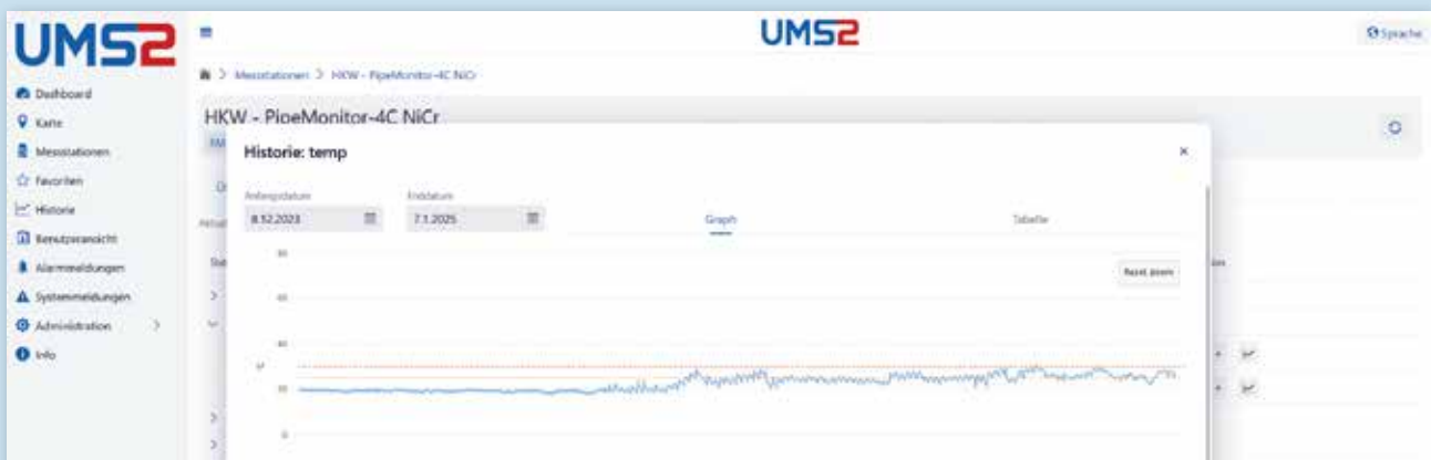
Example of measured value history with pre-alarm (yellow) and alarm limit (red).
