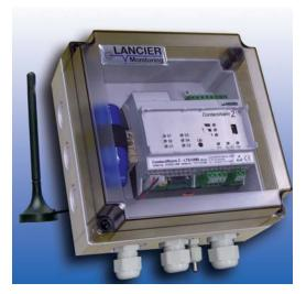
If a contact changes its condition or temperatures\* are beyond thresholds the **ContactAlarm2 LTE/UMS** sends an alarm message to the UMS server via mobile data connection. A weekly status message is always sent, which reports the condition of the equipment. There will be no remote contact surveillance between the measurement cycles.
