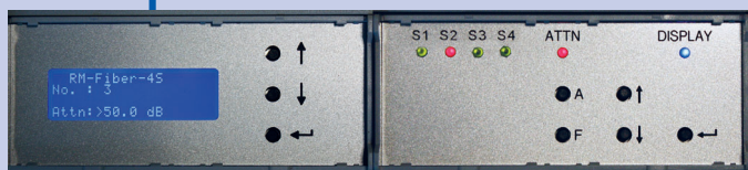
Monitoring station with measuring module RM-Fiber 4S
