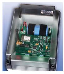
As a LoRa node, the *PipeSens* sensor measures the insulation and loop resistance of surveillance pairs in the insulation layer of district heating pipes on a daily basis, both in the Nordic, hierarchical and NiCr system, thus ensuring monitoring according to **EN 14419**.
