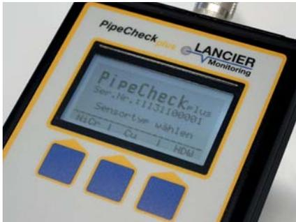
Small, light and efficient: the **PipeCheck<sub>plus</sub>** mobile measuring device by LANCIER Monitoring is used for inspecting existing or newly installed measurement sections in district heating pipeline monitoring.
