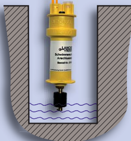
Manhole monitoring - e.g. floating switches with reed contacts
